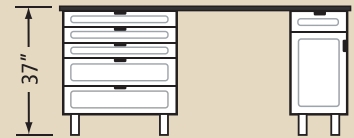
80" Island Workbench Drawer and door units with knee hole 24" depth
